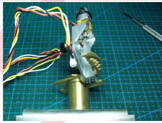
Install gear box assembly / tilt gear components on the bracket with 2pcs M2 * 8 screws.
