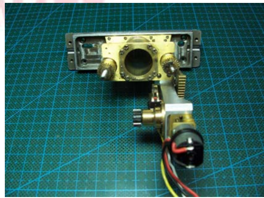
Install shock absorber tube; the right one with resistance device, equipped with E ring.
