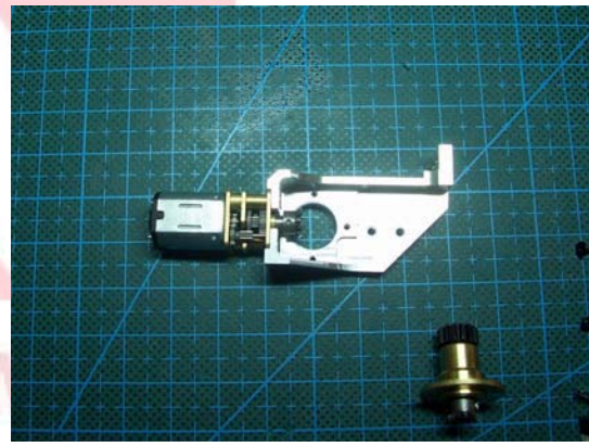
Fix the motor with 2pcs M1.6*3.5
