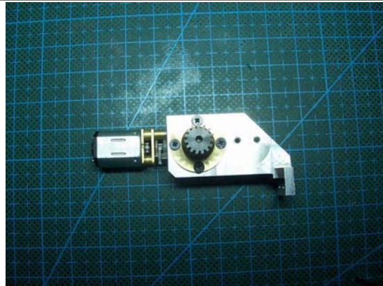
Fix gear components with 4pcs M1.6*3.5
